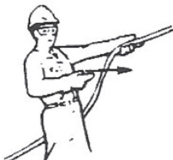
RETRACT BOOM: One-hand signal: One fist in front of chest with thumb pointing outward and heel of fist tapping chest.
