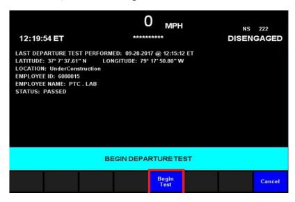
Brake application will perform. <u>Do Not</u> press the fail test key.
