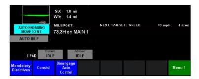
**Auto Control** is now engaged and will control the throttle and dynamic brake.
