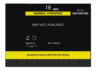
If Restricted Mode is no longer required you can exit while stopped by pressing 'Restricted Mode Off' key, then 'Yes' to Confirm
