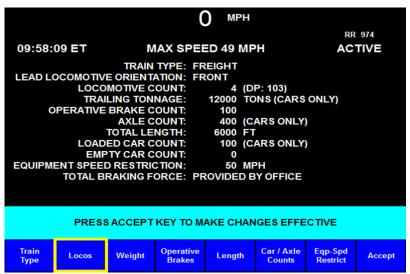
The locomotive position, count and orientation should always be checked before departure for accuracy
